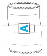
Example: When embroidering a T-shirt Rotate the pattern 180 degrees. Pass the machine bed through from the waist of the T-shirt, not from the neck, and attach the embroidery frame to the machine. Prevent the neck to be stretched when the embroidery frame is moved.
